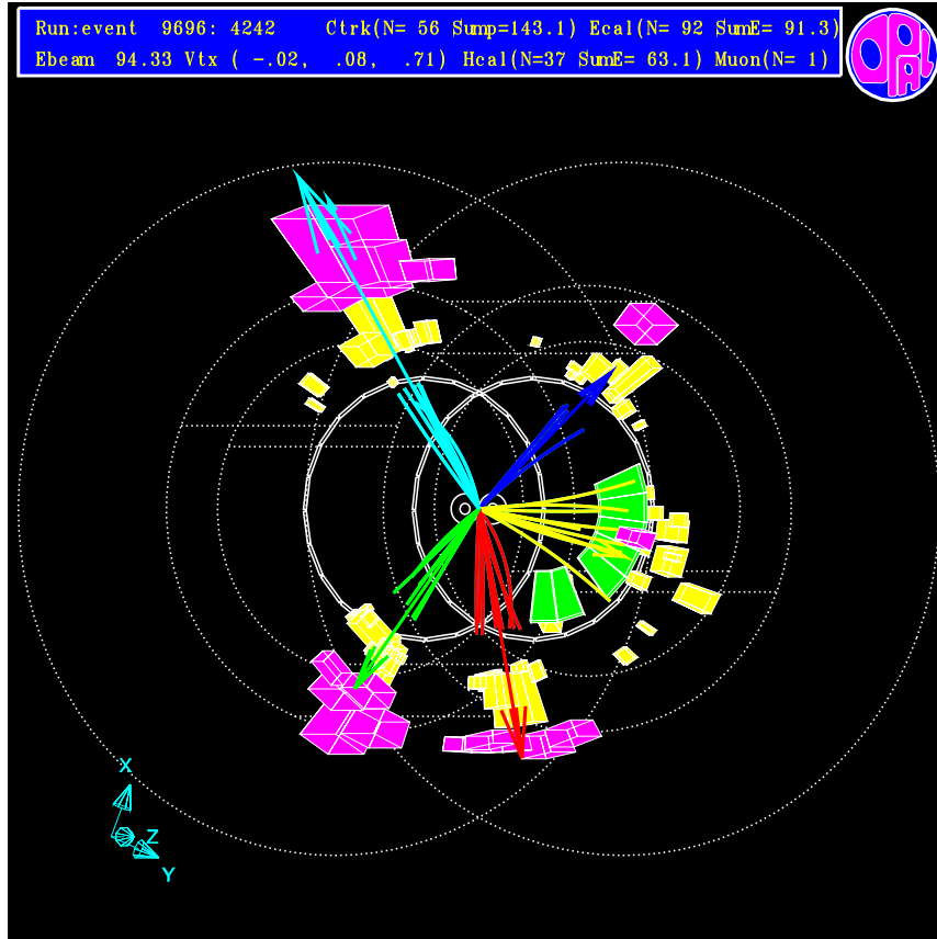
Figure 4.5: A 5-jet candidate recorded with the OPAL detector. This event, although it clearly looks like a 5-jet event ( \ln y_{45} = -4.20 ) with a 5-C fitted mass of M_W^{5j} = 79.43 GeV, it also leads to a reasonable 4-jet reconstruction with M_W^{4j} = 79.20 GeV. The jet pairing likelihood is 0.78 and 0.65 for the 5- and 4-jet reconstruction (see section 4.4.3). Treated as 4 jets, the green and the red tracks, together with their associated calorimeter clusters, would be combined to a single jet.
