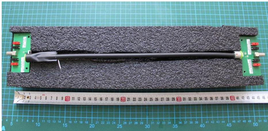
**Figure 10.7:** The SiPM-Fiber prototype with 35 cm long fiber and optical shielding. The SiPM was centered and glued to a plastic structure. A silicone fluid connects the active surface of the SiPM and the fiber.
