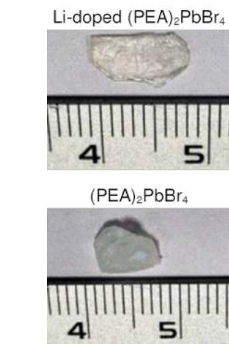
Figure 6.20: Photographs in ambient light of single crystals of Li-doped and undoped (PEA) 2 PbBr 4 , irregular in shape and thickness. Figure adapted from Cala', Frank et al. [36].
