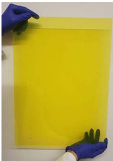
Figure 4.9: CsPbBr 3 perovskite nanocrystals in a polymer in ambient light. Figure from Erroi, Frank et al., [27].
