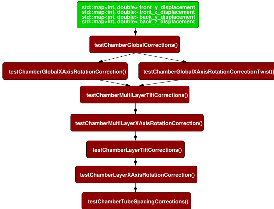
**Figure B.1:** Work-flow of the wire displacement determination software, with variables and methods described in the text. Methods for a global x-axis correction can be interchanged, depending on whether a correction for twisted chamber ends should be performed or not.
