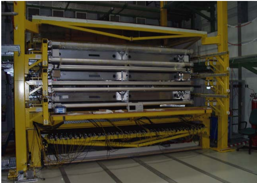
Figure 2.1: Side view of the cosmic-ray test-facility with a complete three-chamber setup.
