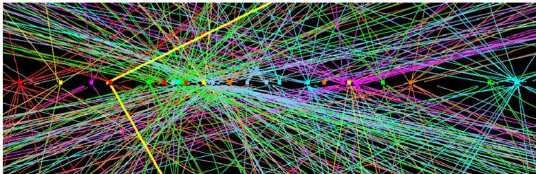
Figure 17: Example of an event display showing in-time pile-up. The dots are the extrapolated tracks of particles to the vertex issuing from inelastic collisions within the same bunch-crossing (from [34]).
