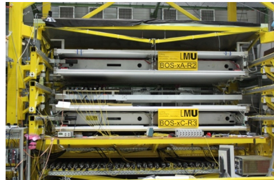
(b) MDT chambers with GEM and trigger scintillators between the MDT chambers and the upper and lower scintillator hodoscopes
