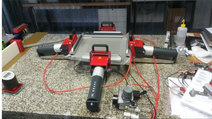
**Figure 9.3:** Photo of the Sefar mesh stretching setup
