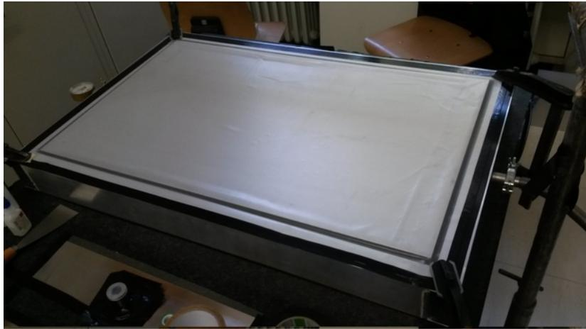
**Figure 7.15:** Evacuated frame with plastic foil to equalise the pressure on the stiffback during curing
