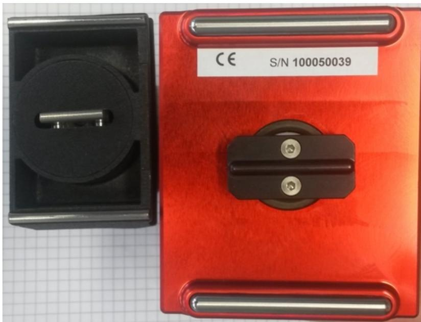
**Figure 9.12:** Bottom view of the Newman tension meter and the Sefar Tensocheck 100; both tension meters have two parallel stationary bars at the borders, and a smaller movable one in the middle; because of this setup it is possible to obtain tension measurement data in the direction perpendicular to the footings
