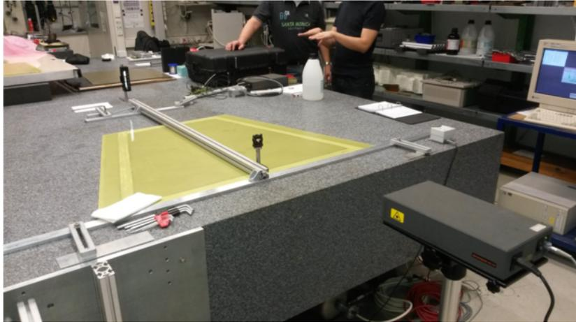
**Figure 6.5:** Experimental setup for an interferometer measurement. The ML10 laser is in the right bottom corner, the straightness interferometer in the middle at the beginning of the guiding bar and the reflector is in the left top corner at the end of the guiding bar. The guiding bar is the aluminium profile in the middle of the trapezoidal area.
