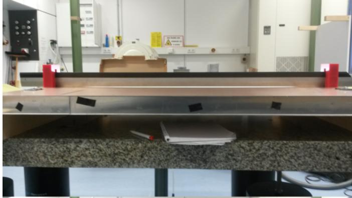
**Figure 7.2:** Bending of the stiffback under its own weight. The airgap is visible by the shining through light.
