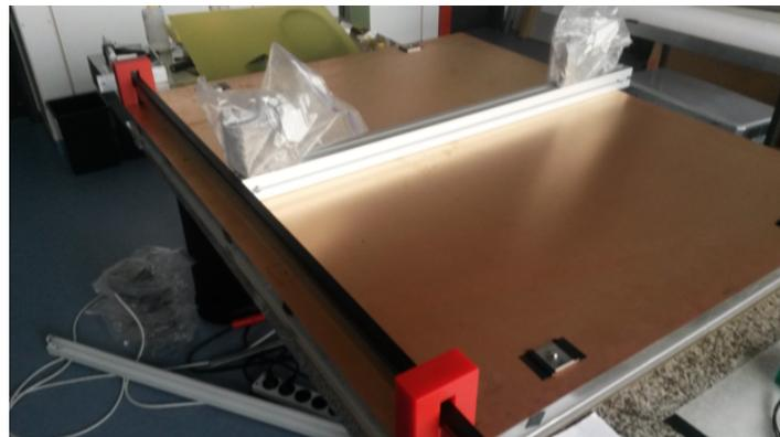
Figure 7.4: Setup for the beam bending experiments of the stiffback
