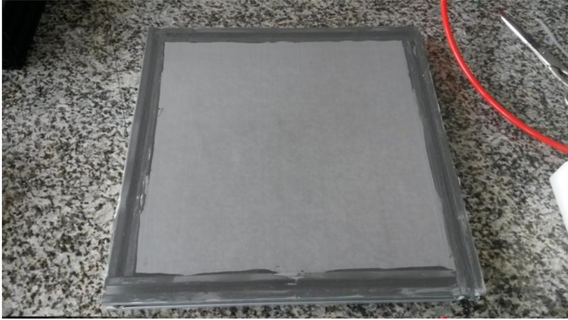
**Figure 9.5:** Photo of a stretched mesh glued onto a  $28 \times 28 \text{ cm}^2$  aluminium frame
