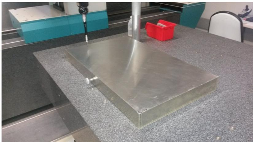
**Figure 7.16:** A 50 cm × 83 cm stiffback in final design layout during a surface scan using a CMM
