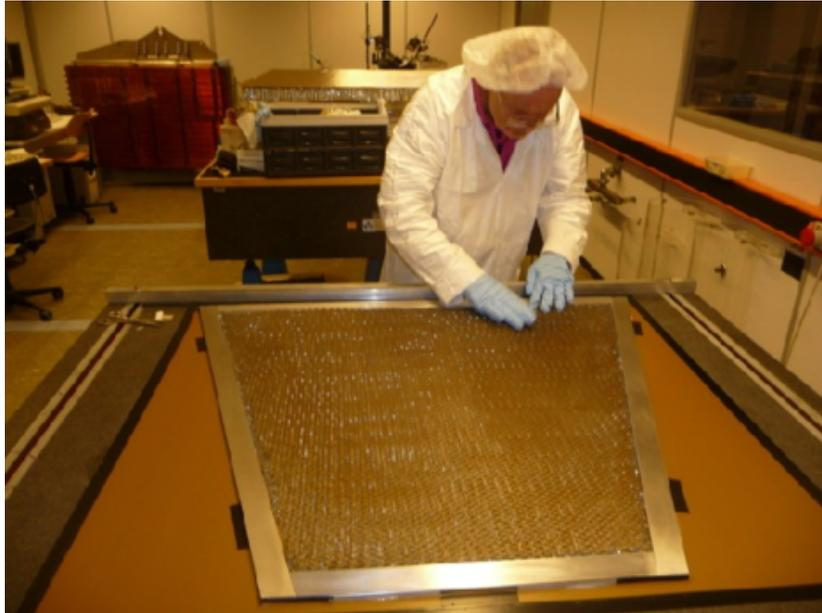
**Figure 5.4:** Photo of the glueing of the first side. The aluminium bars and the honeycomb are already on the FR4 sheet. Photograph taken from [Hertenberger, 2014].
