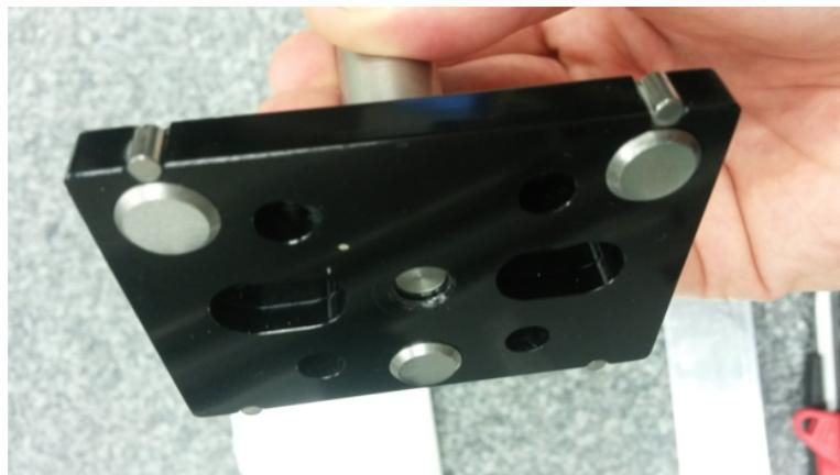
**Figure 6.10:** Tripod pedestal of the interferometer
