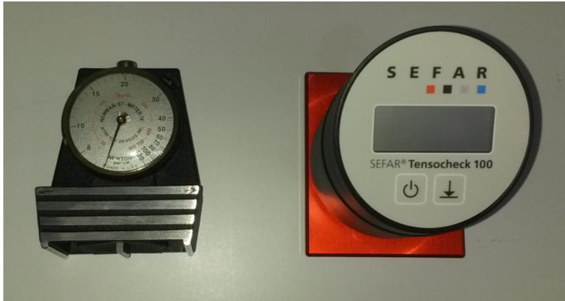
**Figure 9.11:** Photo of the Newman and Sefar tension meter
