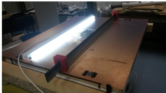
**Figure 7.7:** Experimental setup for measuring the stiffback deformation
