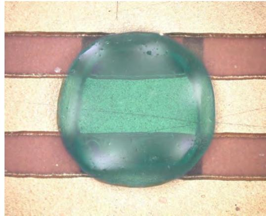
Figure 5.1: Pillar-shaped spacer structure in the active area on the surface of the anode to hold the micro-mesh at a constant distance of  $150\ \mu\text{m}$  to the anode. They are made of solder resist, created with the stripping method and arranged in a raster of  $38 \times 38$  pillars. 2% of the active area is covered with pillars (left). A photograph of a pillar with a diameter of 0.8 mm taken under the microscope (right).
