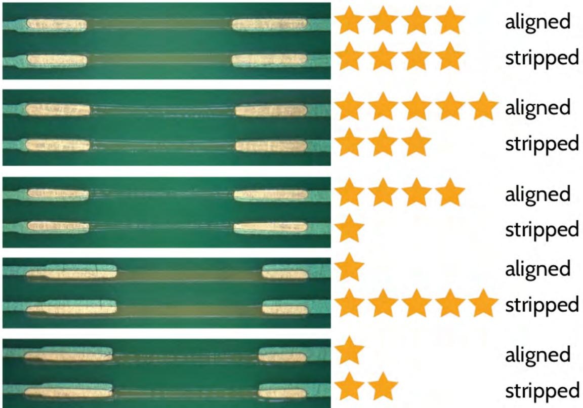
Figure 4.5: Different results of the stripping method, stars rate the results. In order to accept the support structure the following criteria have to be fulfilled: The exposure mask needs to be well aligned with respect to the anode strips. The solder resist needs to be well attached to the PCB and did not soften nor detached from the PCB. The gaps need to be opened up well. The two examples on top were accepted.
