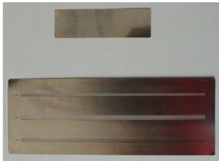
Figure 4.11: Tools for the screen printing method: stainless steel stencil (bottom) and squeegee (top). The  $60 \mu\text{m}$  thin stencil has three different gap widths where the width of  $0.2 \text{ mm}$  is used to apply the paste on the PCB.
