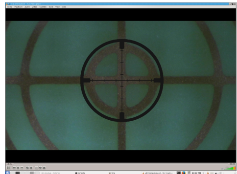
(b) Screenshot of the video signal from a microscope focussing a precision marker on a readout PCB with a crosshair.
