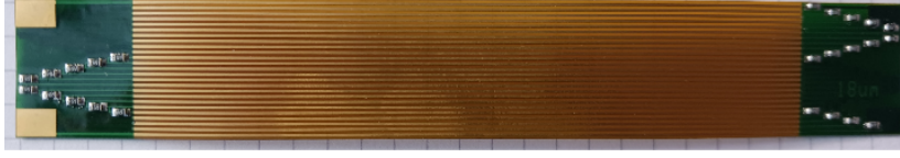
Figure 4.6: Picture of 100/18 conversion layer made of Kapton-like polyimide. 100/35, 50/35 and 50/18 look very similar.
