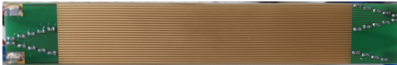
Figure 4.5: Picture of 1550/35 conversion layer made of FR4. 300/35 layers look almost the same.
