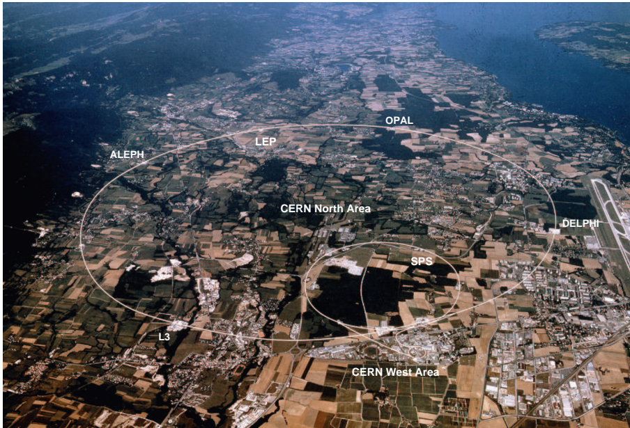
Figure 2.1: Aerial view of the European research center for elementary particle physics CERN. The position of the accelerators SPS (Super Proton Synchrotron) and LEP (Large Electron Positron Collider) with its four experiments ALEPH, DELPHI, L3, and OPAL has been added.
