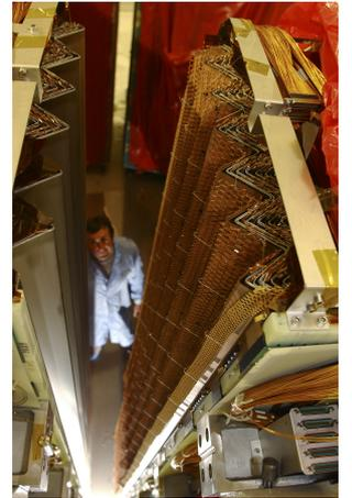
Figure 3.9: Image showing a section of the ATLAS EM LAr calorimeter with the characteristic accordion structure. The picture is provided by CERN.
