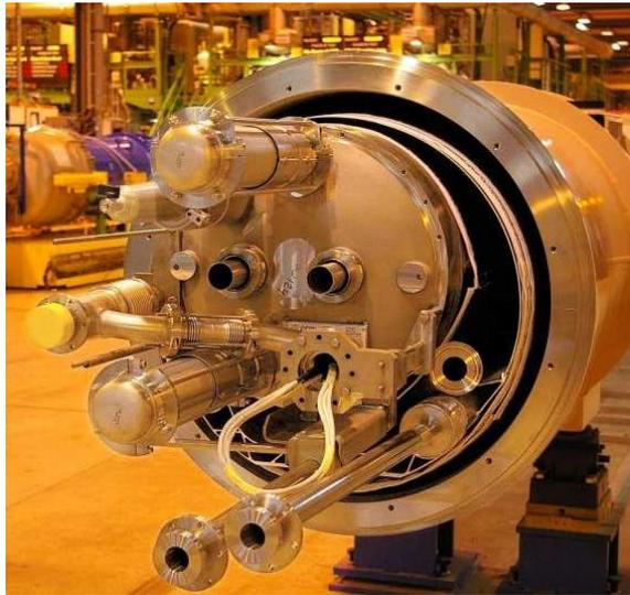
**Figure 3.2:** Illustration of the  $15 \text{ m}$  long LHC cryodipole.
