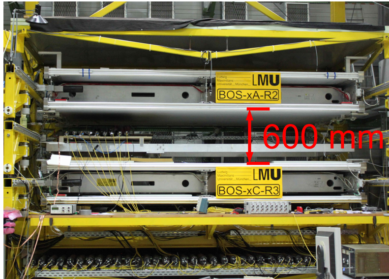
Figure 6.1: Photo of the LMU Cosmic Ray Facility in Garching. The CRF consists of two Monitored Drift Tube (MDT) chambers, two spare chambers for the ATLAS Muon Spectrometer, sandwiched by two trigger hodoscopes. In between the MDTs a 1\text{ m}^2 large Micromegas detector is installed for the calibration.
