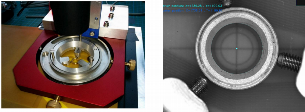
Figure 5.11: Left: Telecentric camera with x-y-manipulator for the positioning of the precision washer. Right: Picture of the precision washer aligned to the circular marker on the PCB taken by the telecentric camera.
